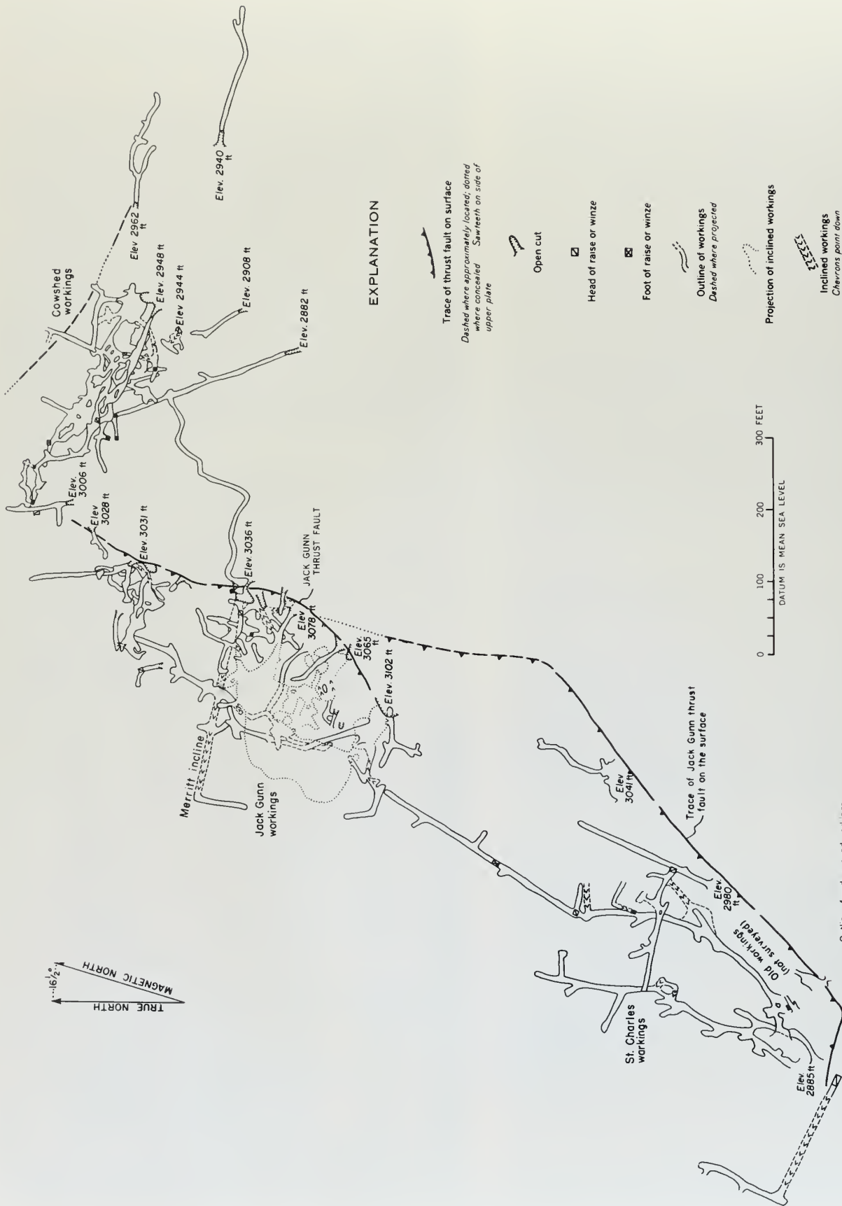
Figure 2. Composite map of the underground workings of the Minnietta mine, Inyo County.
